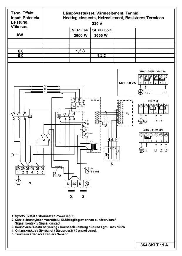
Image 7 Switch diagram for the sauna heater
