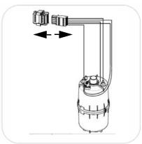
Separate connection plug from heater element harness
