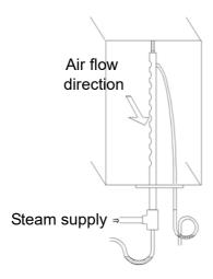
Horizontal installation of the steam manifolds is preferable. However, vertical installation into the air duct from below is also possible.
