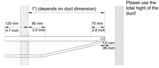
\*) s. table of manifold lengths Horizontal assembly position in duct
